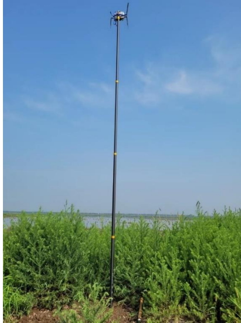
Figure 14. Surveyors tried to receive signals from the satellite-tagged Nordmann's Greenshanks by setting up a Bluetooth hub manufactured by the Druid Inc. Photo by Ziyou YANG
