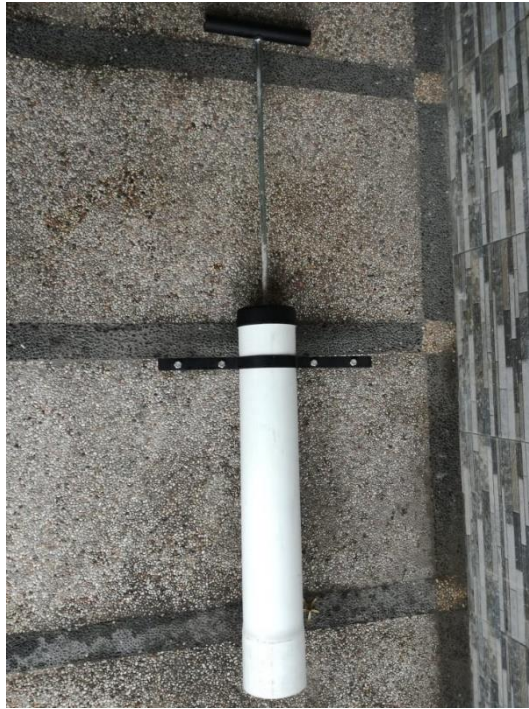
Fig. 02 : Corer. Tool that used to take benthos sample.
